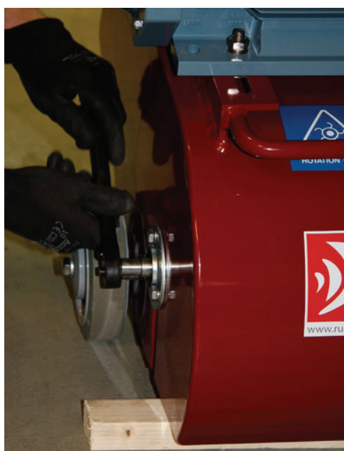
7. Remove bolts on the other side of the chassis and loosen the allen screw (*fig.1) like picture above.
